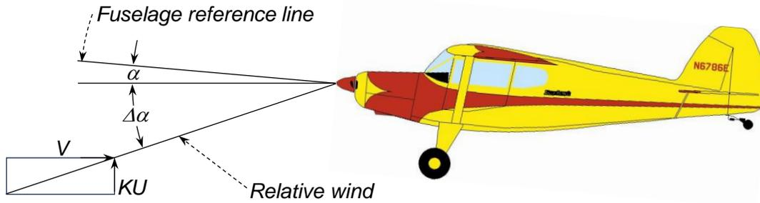
We will use the small angle assumption that  $\alpha = \tan \alpha$  for small angles (as measured in radians). Therefore, the incremental change in angle of attack can be expressed as
